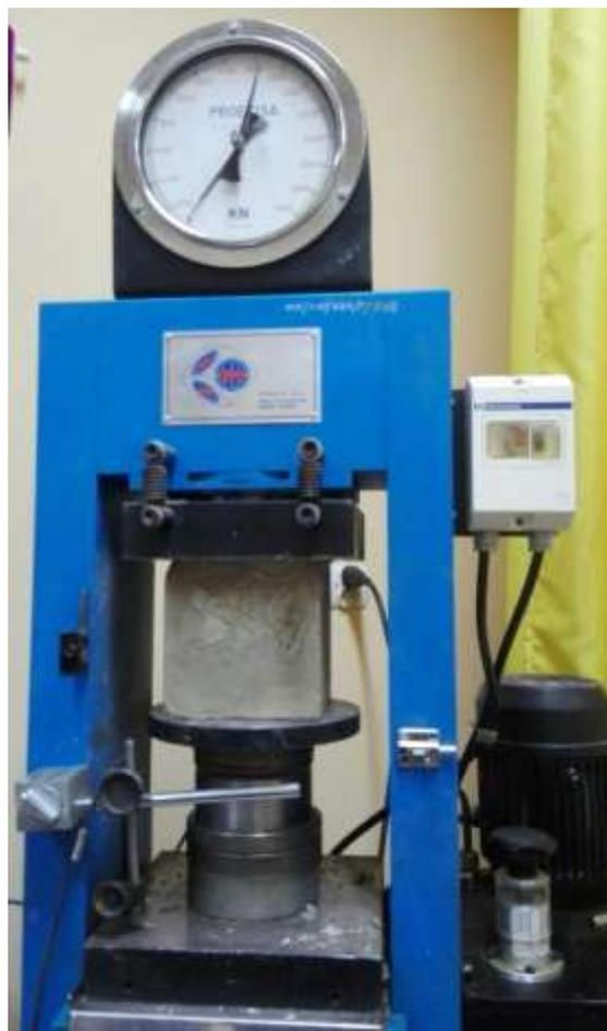
Fig. 3. PROETI testing machine
