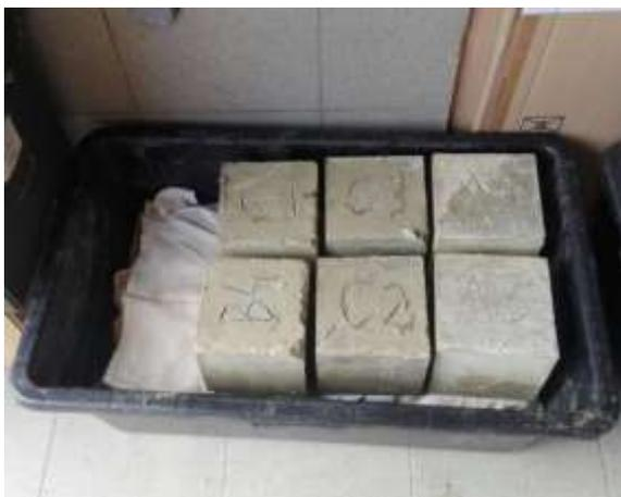
Fig. 2. Samples after unforming
