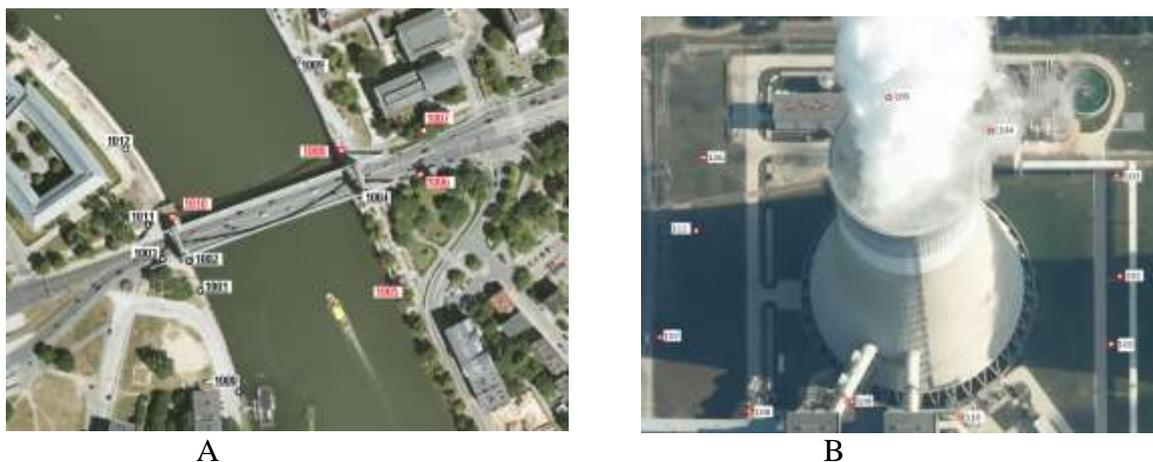
Fig. 1. Sketch of the distribution of the control points around the objects: A) around the bridge and B) around the cooling tower (source: ortofotomap: <http://maps.google.pl>)
