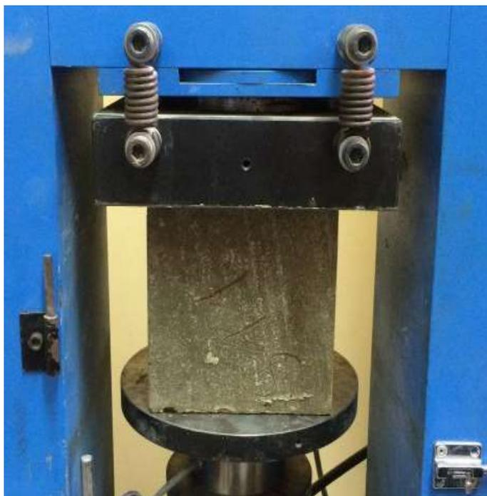
Fig. 1. Cubic sample of cement-soil in PROETI testing machine
