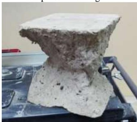
Fig. 4. Example of samples destroyed (tested) one week after preparation
