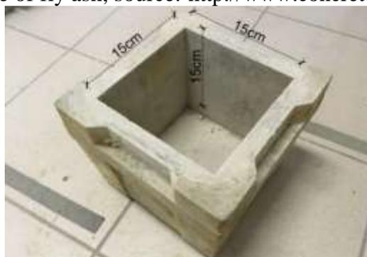
Fig. 2. Cubic mould for concrete soil-cement sample
